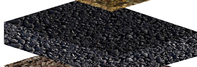
70mm (min) Open Binder Course Asphalt AC20 open binder. Max 100/150 pen to BS EN 13108-1:2006 bituminous macadam
